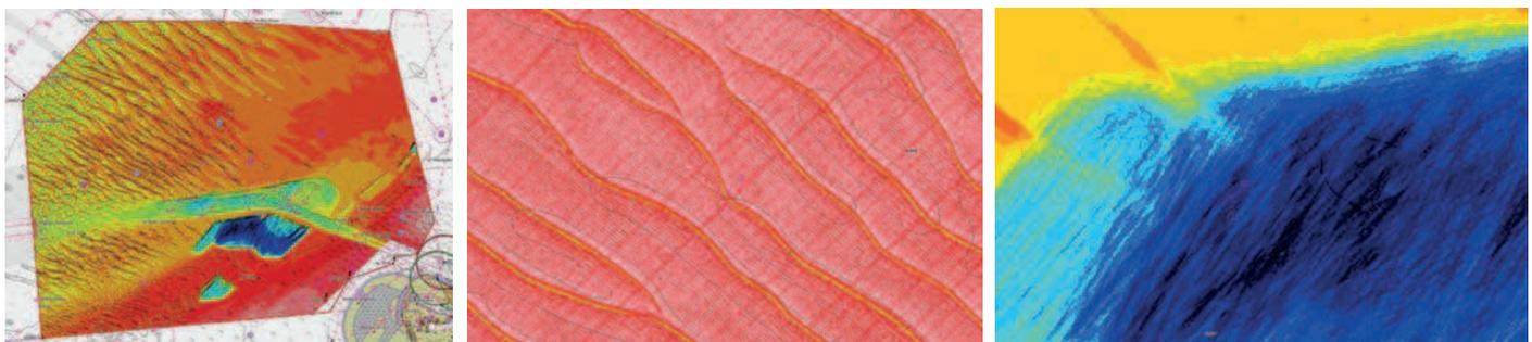
**Figure 2.** Bathymetric data of the May/June 2012 survey of the approach area to the Port of Rotterdam. Overview (left), detail of the sand wave field (center), detail of the main sand pit (right). Notice the small megaripple pattern superimposed on the sand wave pattern, and the dredging tracks in the sand pit. [figures courtesy of crew HNLMS Snellius, Netherlands Hydrographic Service]
