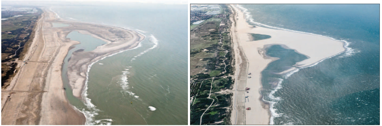
Figure 3: morphological development of the Zandmotor: situation of January 2012 (left) and May 2012 (right) 10
